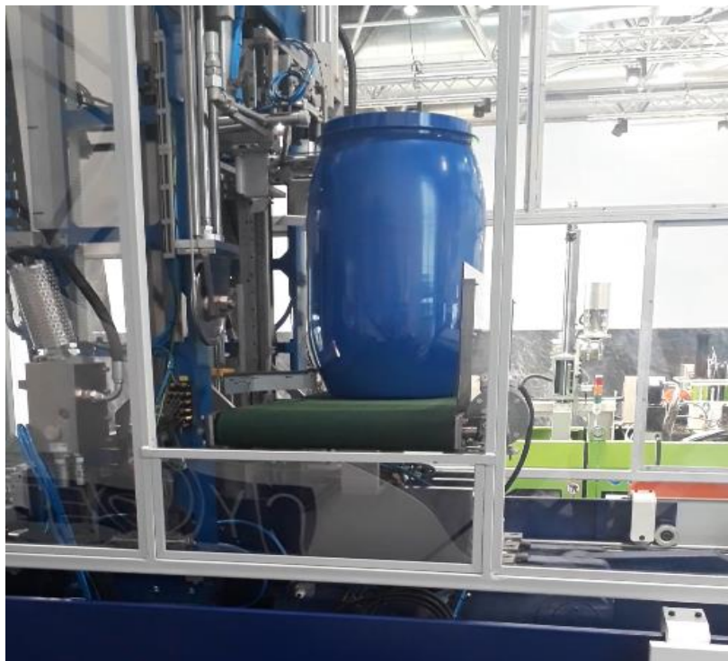
120Ltr PET Drum Production on a CYPET machine at K 2019
